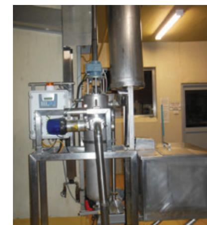
New honey straining system prior to storage
