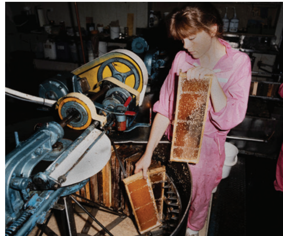
Hand loading fully automatic radial extractors
