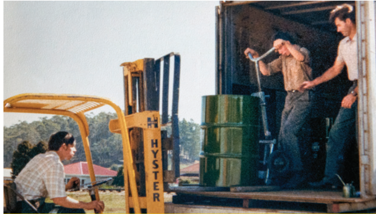
Fork lift loading 300kg drums with barrow assistance for Germany
